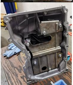
Reinstall all the bolts and windage for final assembly.
