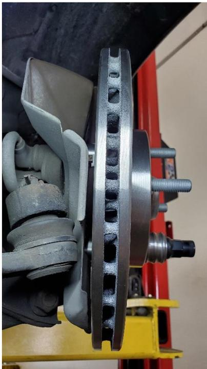
4) Clean off hub surfaces where the rotor will sit - applying a bit of anti-seize compound around the hubcentric area doesn't hurt either. Then, install the new ND rotor and secure it hand-tight with a nut & collar/washer to seat the rotor flush in preparation for caliper installation in the next step.
